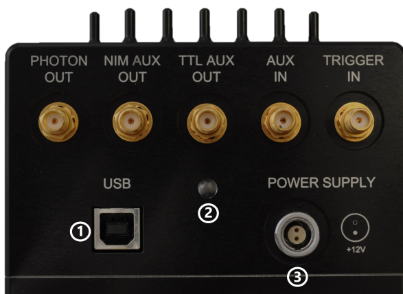
Figure 5. PDM-IR rear panel with highlighted connectors.
